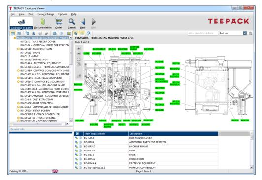
Assembly tree Drawing Parts list The window is structured so that the assembly structure is shown on the **left** as a **tree view** and next to it the **drawing** and **parts list** of the selected assembly can be seen.
