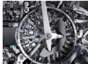
The "heart" of the PERFECTA machine. Continuously working transport wheel with the stations forming the filter paper bag
