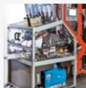
**Integrated box erecting device type ISA and integrated lid closing device type IDS**
