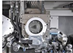
Dosing station with dust exhaust device and filter paper tube forming station
