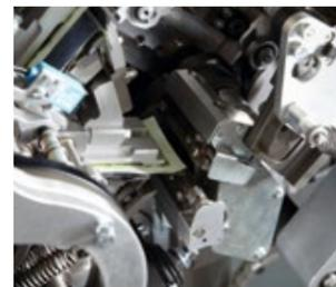
Sealing jaws (heat seal envelope)
