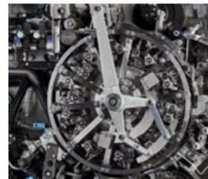
The "heart" of the PERFECTA machine. Continuous working transport wheel with the stations forming the filter paper bag\*
