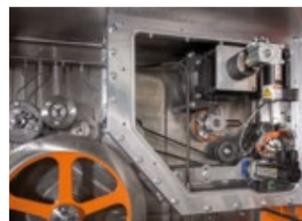
Drive, drive for filter paper and dosing. Motor operated bag weight adjusting mechanism
