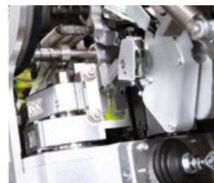
Sealing jaws (heat seal envelope)
