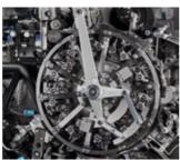
The "heart" of the PERFECTA machine. Continuous working transport wheel with the stations forming
